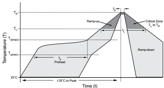
**Note:** If the wave soldering temperatures exceed the recommended profile, devices may not meet the performance requirements.
