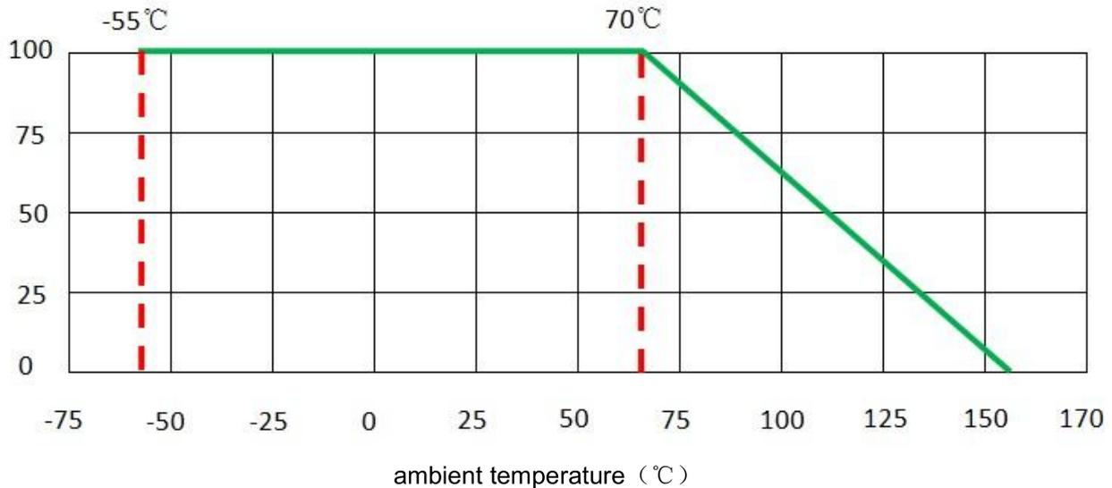
Note : For resistors operated in ambient over 70°C, rated load (rated power) shall be derated accordance With the above figure.
